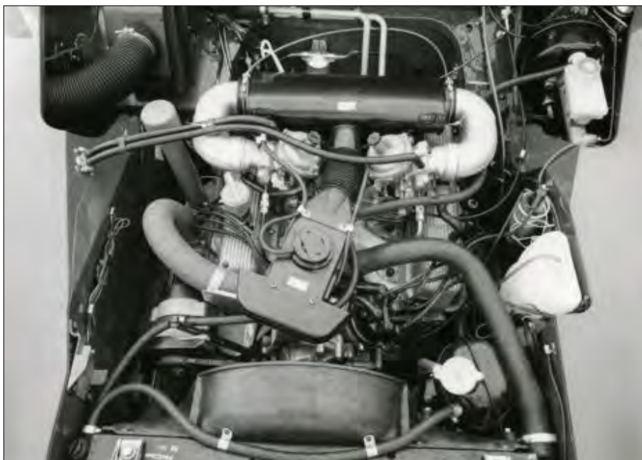
The V8 engine was detuned from its Range Rover application. This was the UK press release picture, although it shows a LHD model.
