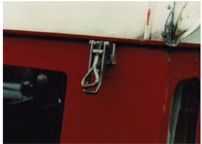
Large over-centre catches, like this one on a late Series IIA model, held the roof shut.
