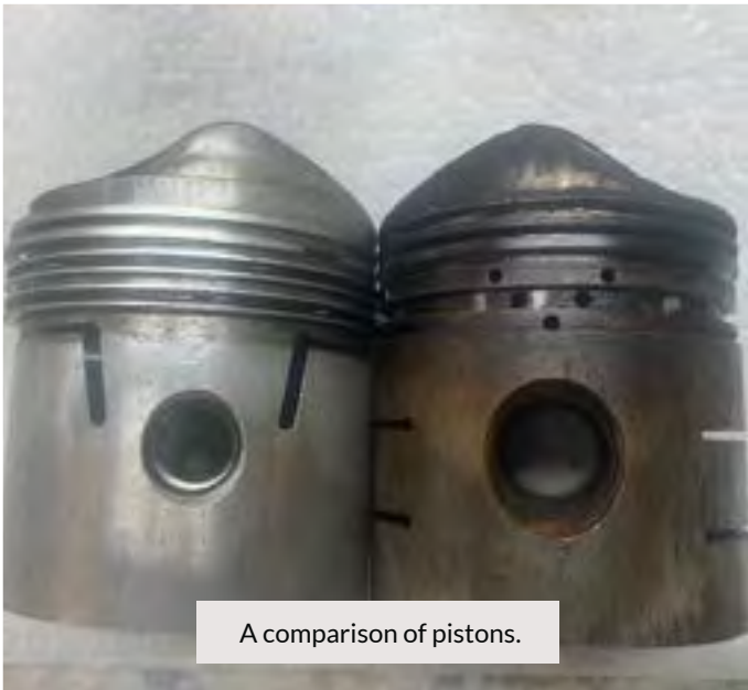
A comparison to early and late gudgeon pins. Mine had the early type.
