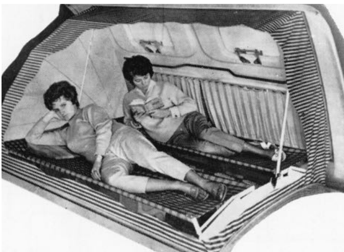
Bunks rolled out at cantrail height to provide sleeping accommodation for two more. This cutaway view was created for sales literature.
