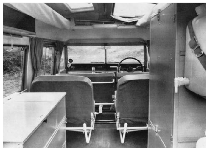
This is the interior of an early Dormobile, showing the Dormatic seats. Later ones did away with the gap between the rear pair.
