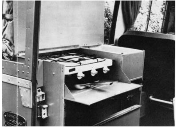
The cooking area was enclosed in a metal box at the rear.
