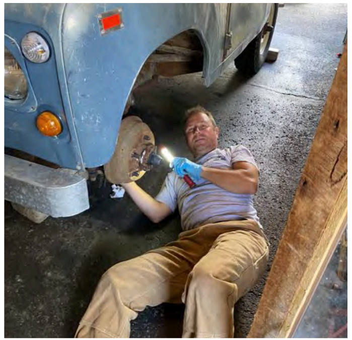
Alastair Sinclair starts the process of changing the swivel ball seals with a thorough cleaning of the hub area to ensure that it is all clean and ready for a swivel oil seal replacement.
