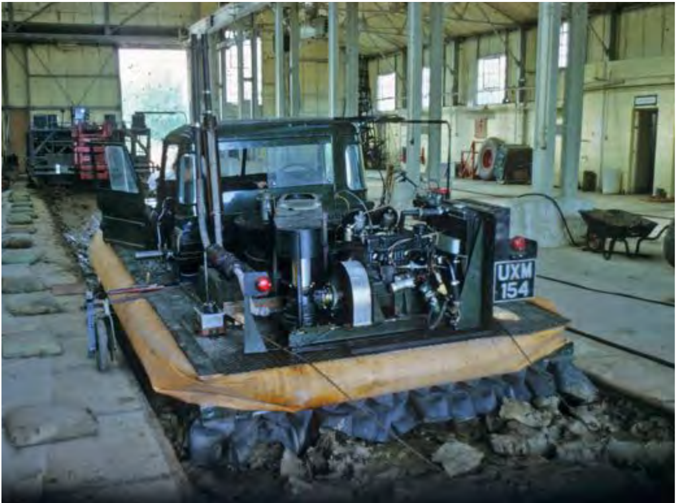
UXM 154, the military conversion, shows how the second engine installation takes up the whole of the rear body space. (6)
