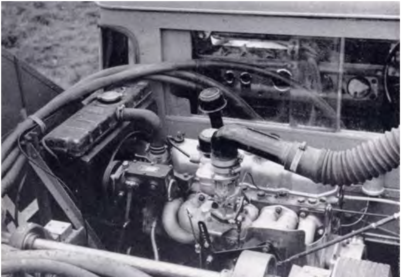
The second Land Rover petrol engine was mounted transversely behind the cab to drive the two fans for the air cushion.
