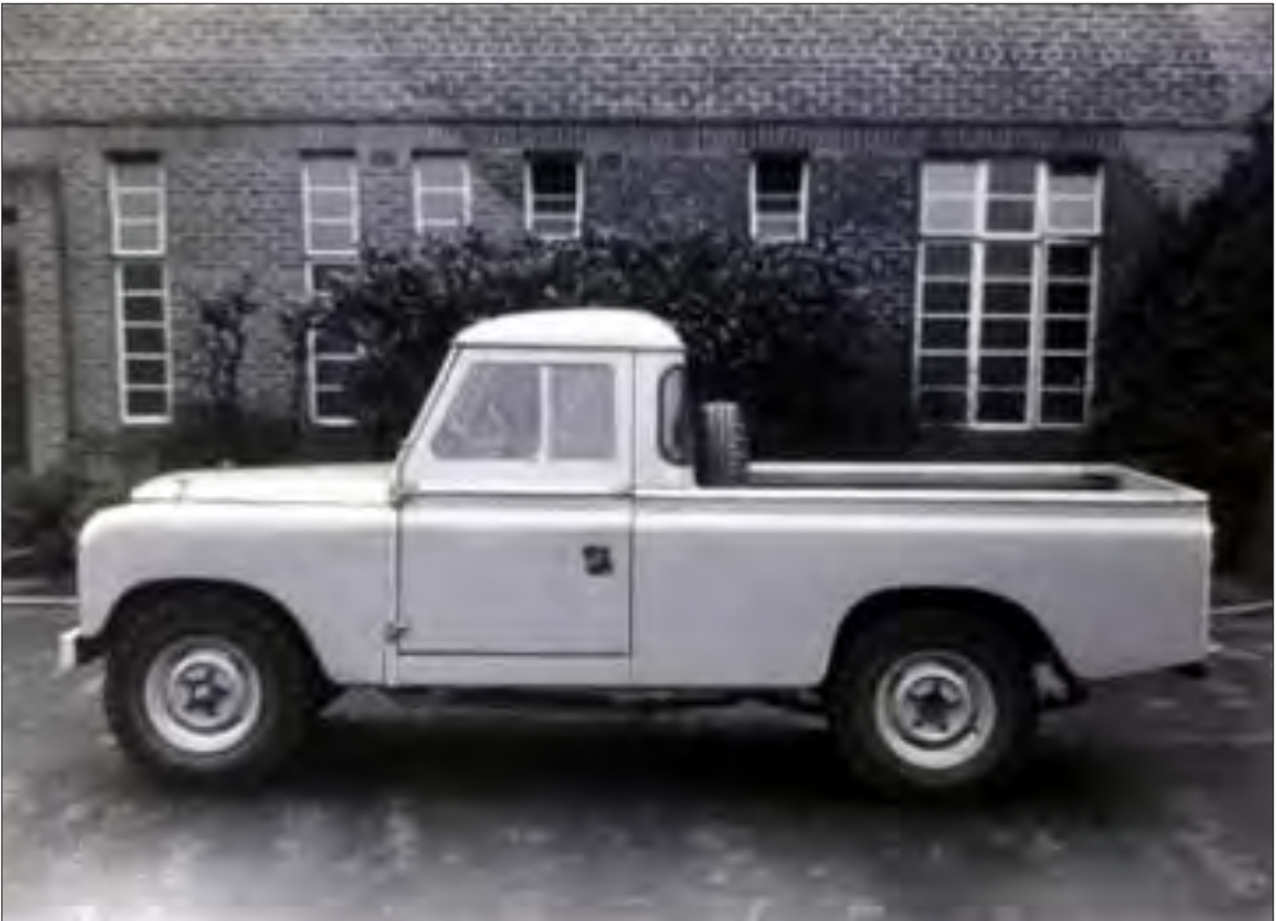
The body on 109/1/S2 seems to have been completed later, adapting styling themes from the Station Wagon. The door window differs from production types, the sill panel is only visible under the door, and the spare wheel is stowed against the back of the cab rather than at the side of the back body.
