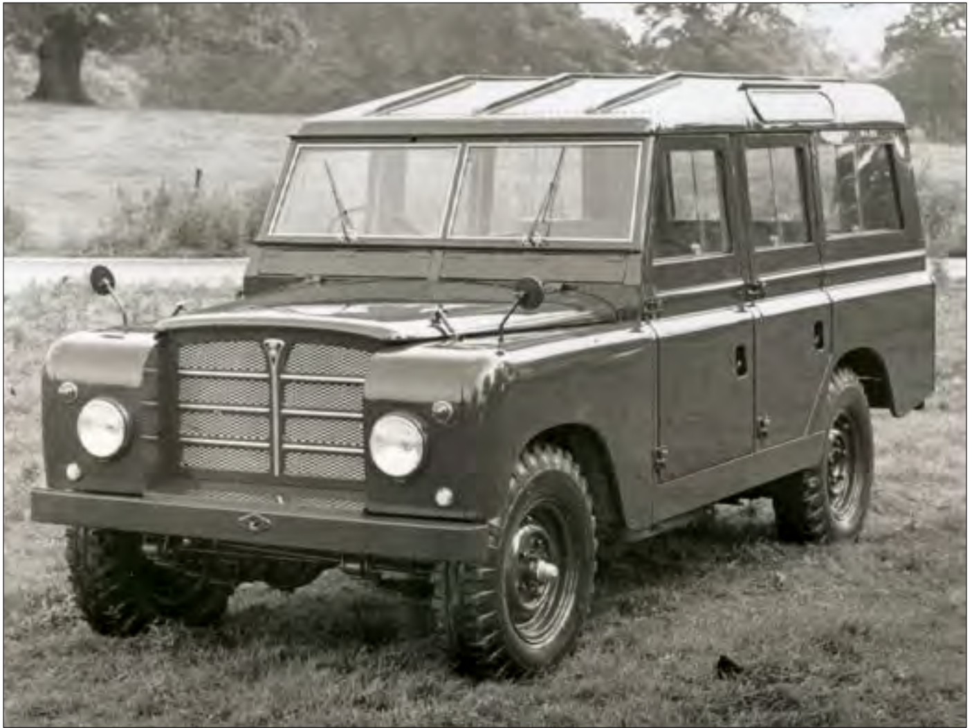
The Daddy of them all. David Bache's prototype body was built on the second prototype chassis, 109/2/S2. That appears to have been a modified 107 Station Wagon chassis.
