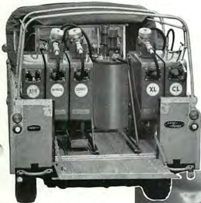
Above: a close-up of Lubrequipment installed on a Land Rover, a good example of one of the compact and efficient installations obtainable.
