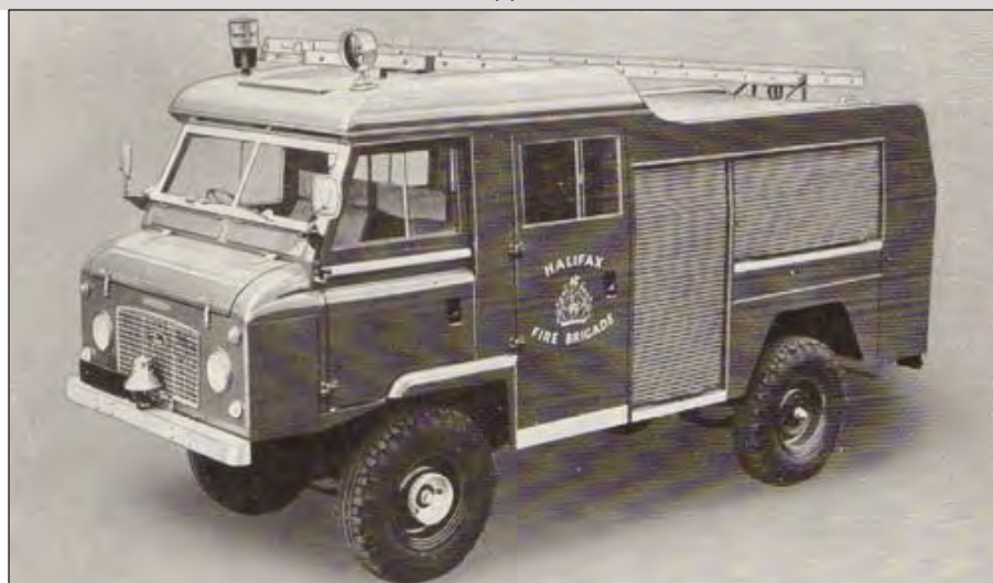
The FT/7 on Land Rover's own Forward Control chassis proved less popular than its rival by HCB-Angus. This one was for the Halifax Fire Brigade.
