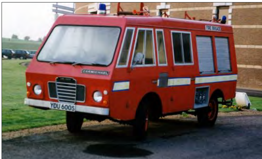
The FT/6 was redesigned with GRP bodywork in the mid-1970s. (Roger Conway photo)
