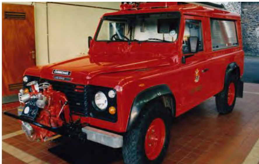
One Tens tended to have front-mounted pumps rather than the traditional Carmichael mid-mounted type. This is a 1987 example.
