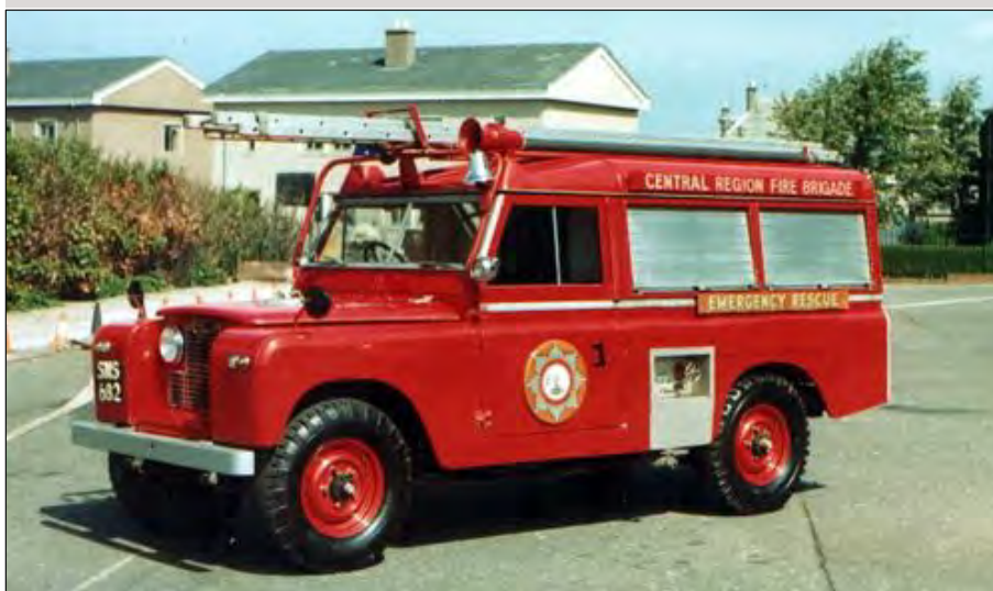
This Series IIA 109 for the Scottish Central Region Fire Brigade had an individual design, but the mid-mounted control panel for the fire pump was typical of Carmichael.
