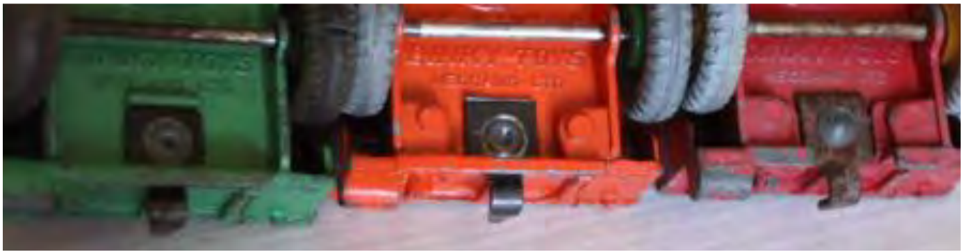
Area of the hook details. On the left green model (V0) with lug in front of the hook. On the centre, orange model with blocks around the injection points (V14). On the right red model with double steps blocks and no more bridge around the hook (V15).
