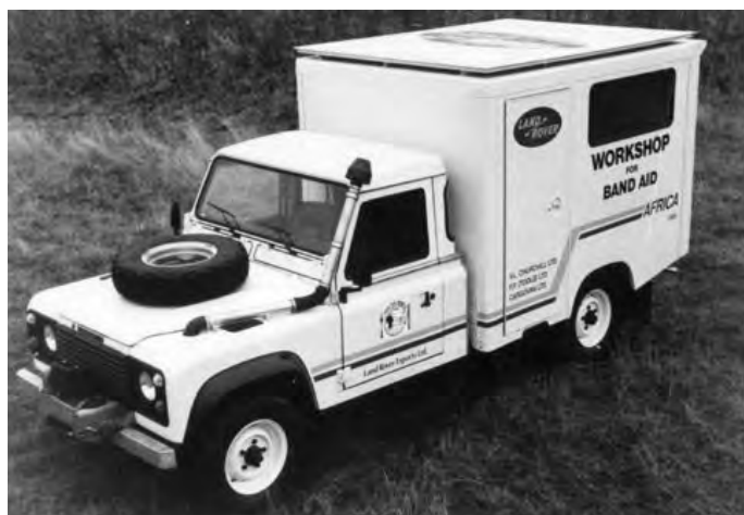
This one will date you if you know what it is! It's a Quadtec body on the 127 chassis, provided to Band Aid for charity work in Africa.
