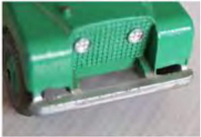
Mask spraying change of front bumper between orange V1 version and green V2 version
