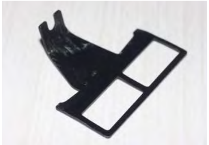
Picture of a dismantled windscreen allowing to see the fork to secure it to the front casting pillar.
