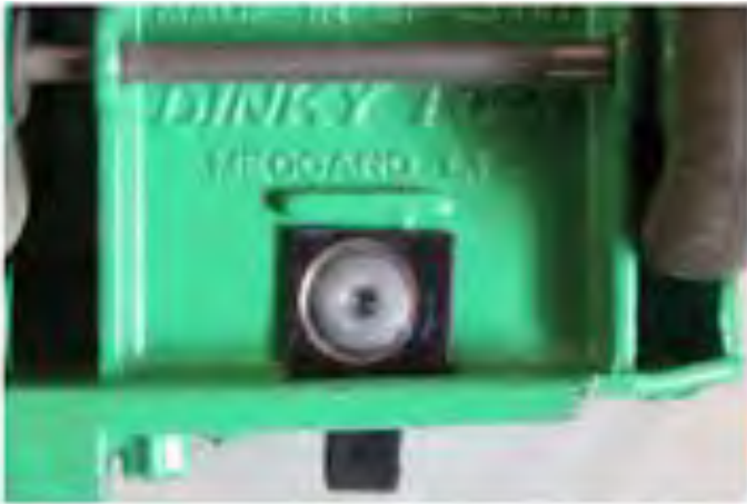
xLug maintaining the rear hook on green V2 version, then deleted on orange V4 version. Note the slight mis-alignment of the hook after deletion of the lug.
