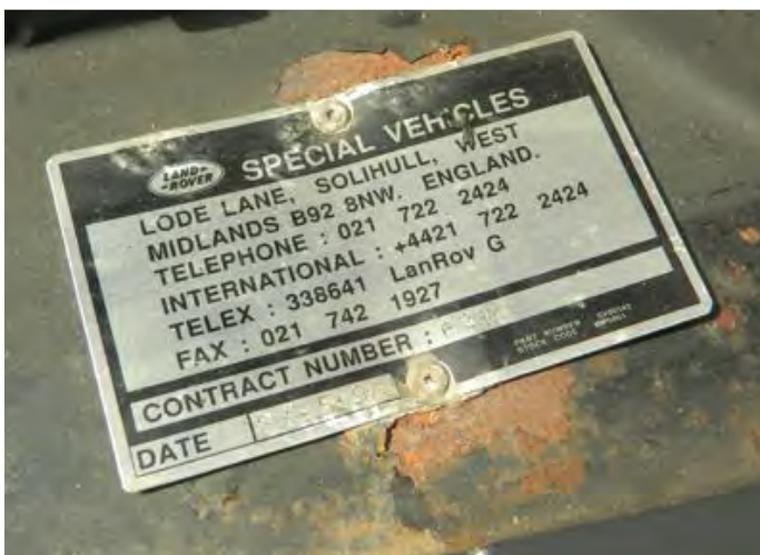
It was possible to reproduce the logo (and some people did), but this one was a bit harder. It's the Special Vehicles contract plate that's found on the bonnet lock platform.
