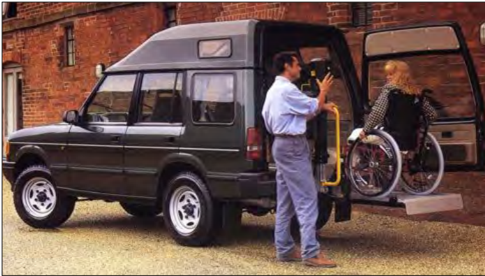
The Discovery wheelchair carrier was a very clever conversion from SVO. Note the raised roof to give headroom.
