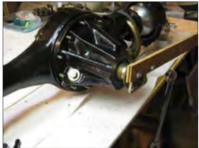
Pinion bearing preload measurement 6-10 in. lb
