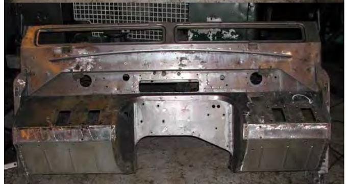
(Figures 21 & 22) Finished firewall in bare metal, ready for coating.
