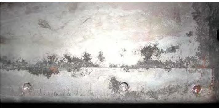
(Figures 4 & 5) Disassembly is the most important part of repairing a firewall correctly. In general try to be as conservative as possible so that the original construction can be replicated when reassembling. The footwell panels are secured with spot welds to the door posts
