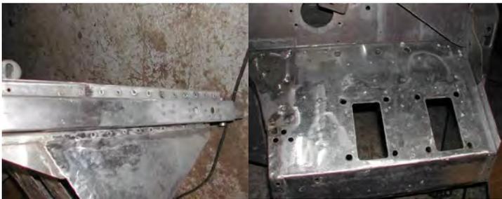
(Figures 17 & 18) With The panels assembled the finish welding can be done to replicate the original construction
