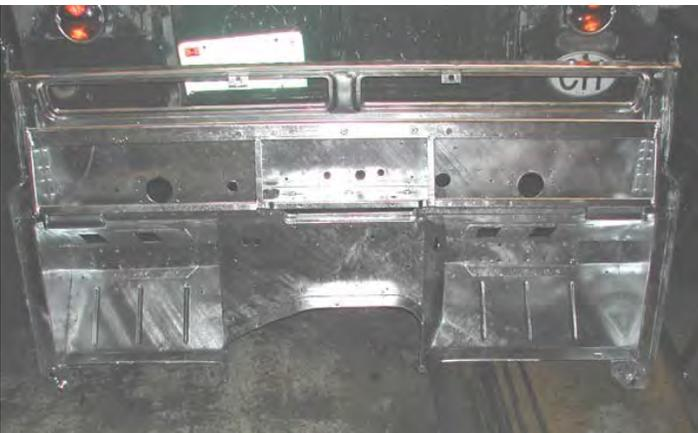
(Figures 1 & 2--above and next column) Here is the completed firewall resplendent in a fresh coat of Hot Dipped Zinc. Ready for fitment to a land rover and sure to last decades longer than a paint job!
