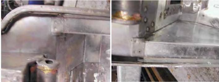
(Figures 14 & 15) Here you can see the small tab which spans the seam between the kick panel and the upper bulkhead. Many times this small detail is deleted. It is easy to retain as its only spot welded to the upper bulkhead and the kick panel slides right in behind it. Noting details like this is the key to repairing the bulkhead in a manner consistent with the original.
