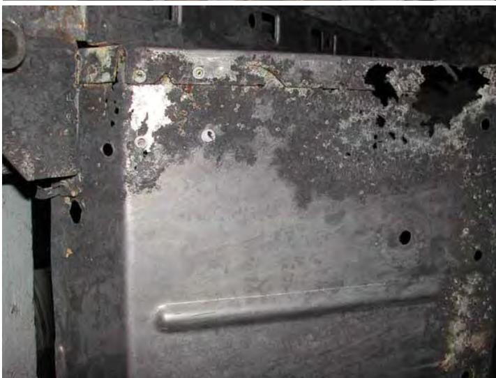
(Figures 1 & 2) This is typical lower bulkhead corrosion requiring the replacement of the toe board and kick panel. It certainly looks ugly but a quality repair here is not difficult.
