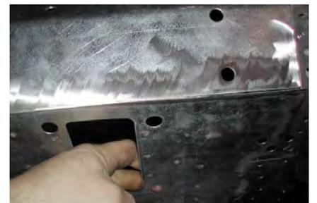
panels overlap, some shops just spot the two together leaving a seam which is not consistent with the original construction. You can do it this way and have a good repair, but we took the extra time for this project to show you how to make it even better. Here you can see that the panels have been trimmed so that they butt up to one another. Even before welding the fit is extremely close. Achieving this sort of fit is important to a good result.
