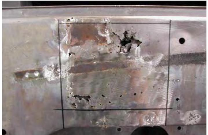
securing the drip rail to the firewall being careful not to drill all the way through the firewall. Drill just enough to detach the spot welds. This is best done with a sharp 3/16 or 7/32 bit at low speed. Take note of how these items are attached so that you can reproduce the welds when reattaching them.
