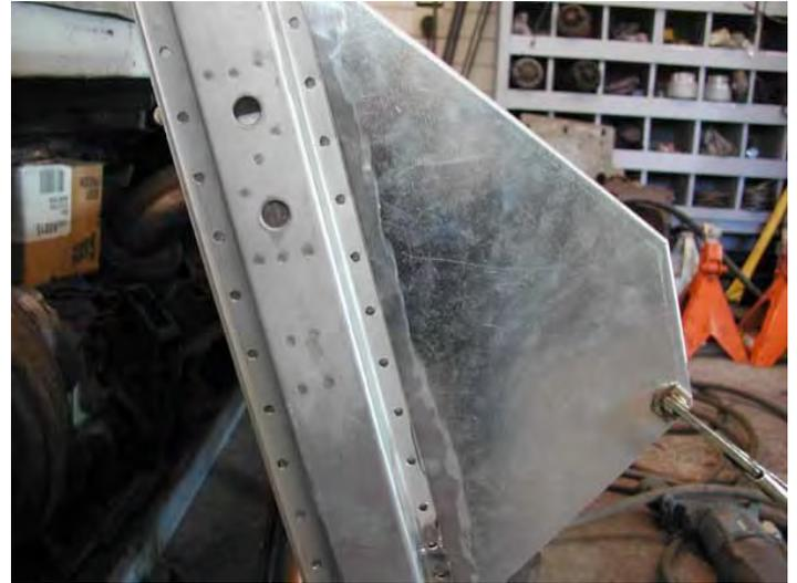
(Figure 11) With the door post accurately replaced the footwell can then be assembled. Here you can see the replacement door post has been drilled and the galvanizing ground away in preparation for welding the two panels together.
