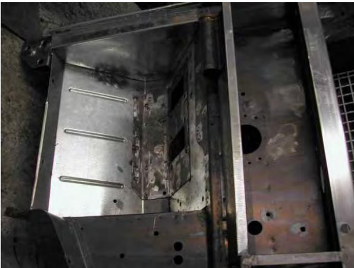
(Figure 16) With the toe board welded to the upper footwell and the kick panel in place, the stiffening panel can then be spotted onto the assembled footwell
