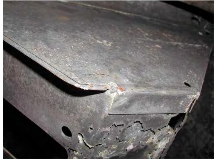
(Figure 6) Take note of construction details during disassembly. Here you can see a small weld securing the upper footwell panel to the kick panel. While this may seem anal to replicate a detail nobody is likely to notice, the goal here is to make an original looking repair, not just fool someone who doesn't know what they are looking at.
