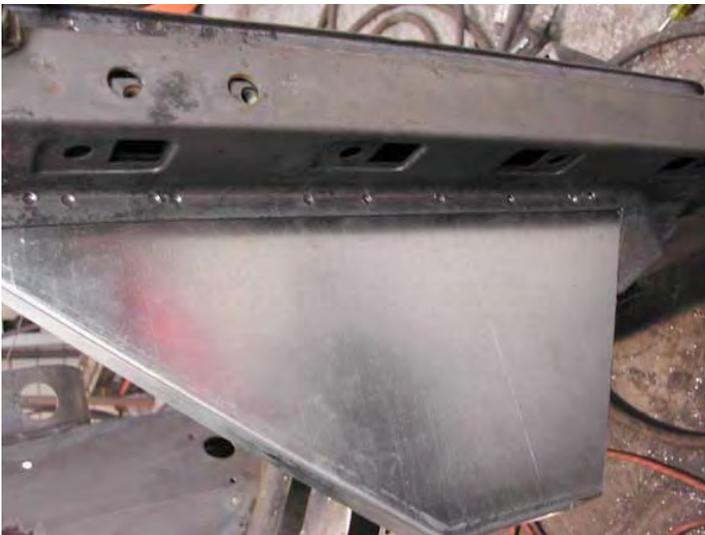
the new panel can be test fitted. You can see that correct removal of the old panel makes reassembly much easier. The stiffening web referred to in the last set of pictures is visible here at the right side of the photo. Since the panels are lightly galvanized, mark the panel where it will be welded on reassembly and grind the
