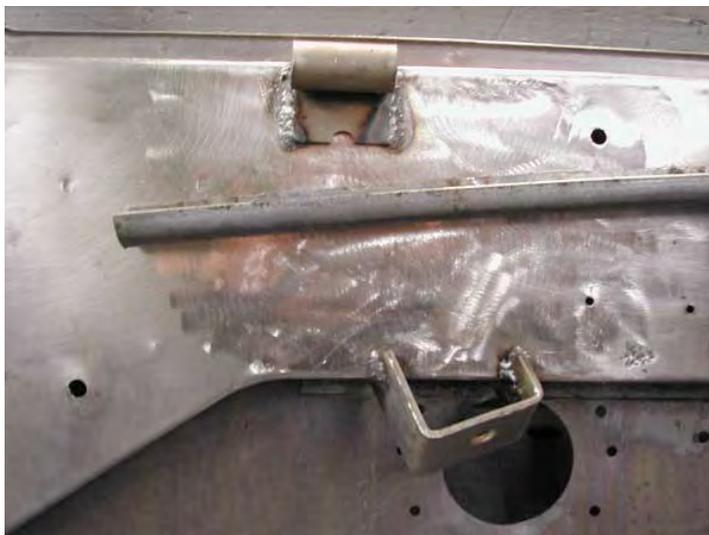
(Figure 4) With the finish welding complete and ground flush, the hood hinge, support bracket and drip rail can be reattached. Refer to the measurements you made earlier to ensure a good fit for the hood. The completed repair will be difficult to spot and once coated will be extremely durable.
