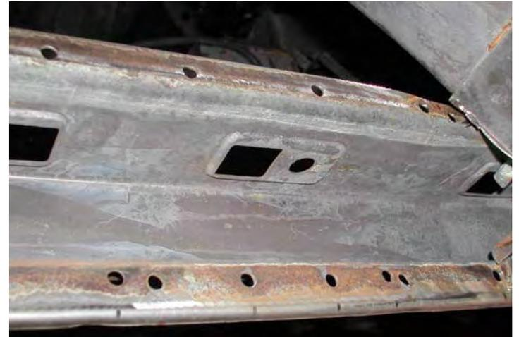
(Figures 7 & 8) Here you can see the doorpost with the footwell carefully removed. Mark the holes that were spot welds to distinguish them from the holes used for riveting the door seal to the seal lip. During reassembly this will allow you to put the spot welds where they belong. Also take note of the two small tack welds in the right
