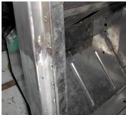
(Figure 10) With the old post cut off the jig is used to position the
