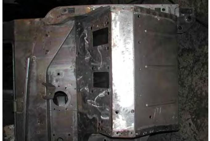
seam welds have been replicated and the firewall is rust free and ready for coating.
