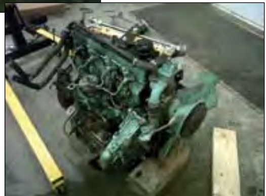
2.5 NA diesel out of vehicle - complete
