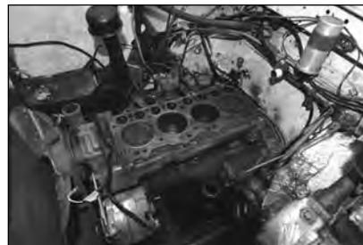
Given this head with the stuck valves would be needing some work, another head was needed. Happily, there was one at hand on the engine that came north from Ben’s in October for the BGB. So, Alastair and I pulled the head off the late
