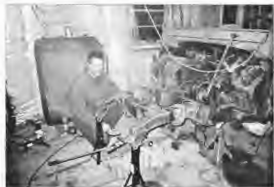
Eureka it fits! Front chassis horns from 88" tacked into place on the front of the 109".
