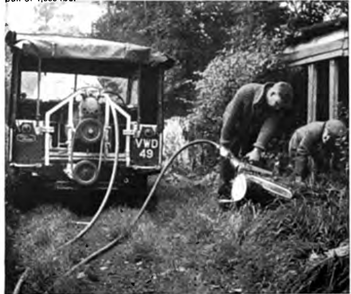
Power plant. When fitted with centre or rear power take-off, the Land-Rover can operate all kinds of specialised equipment—in this case a compressor and pneumatic chain saw.
