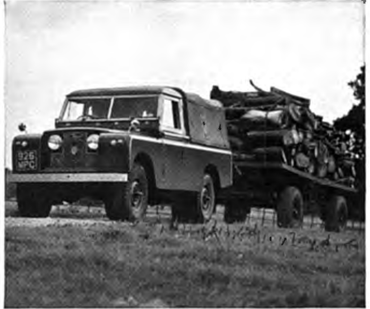
Load-hauler. A regular Land-Rover makes light work of a heavy load. With its powerful 2½ litre engine (Petrol or Diesel) the vehicle has a drawbar pull of 4,000 lbs.
